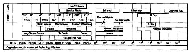
Figure 2-1. Electromagnetic Spectrum
