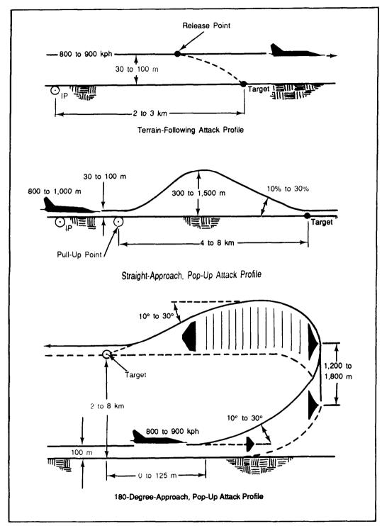
Figure 7-2. Typical Aerial Attack Profiles Against Fixed Facilities
